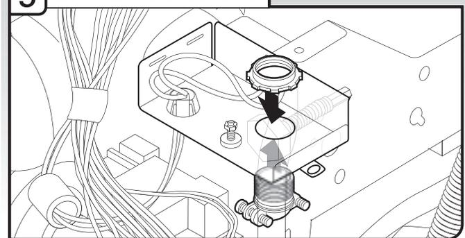
Install a UL Listed/CSA Approved strain relief. Make sure screw heads are facing to the left when tightening conduit nut. Strain relief may be provided with the power supply cord kit.
